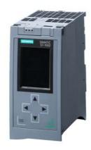
\*\*\* Spare part \*\*\* SIMATIC S7-1500, CPU 1516-3 PN/DP, central processing unit with work memory 1 MB for program and 5 MB for data, 1st interface: PROFINET IRT with 2-port switch, 2nd interface: PROFINET RT, 3rd interface: PROFIBUS, 10 ns bit performance, SIMATIC Memory Card required
